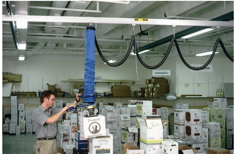
A special suctionfoot, art nr 30620 was developed for the purpose of lifting boxes of wine; heavy, fragile with a small lifting area.
